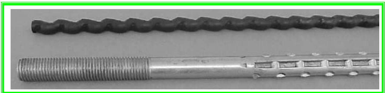
Picture #5: "Mine Roof Bolts"
